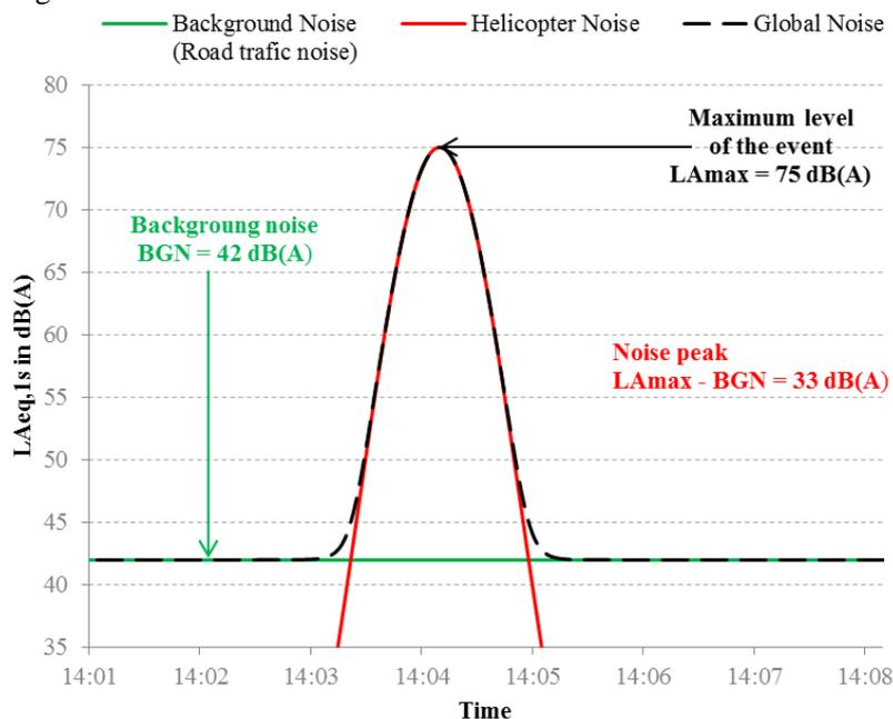
Figure 1 - Example of an "aircraft"-type noise peak
