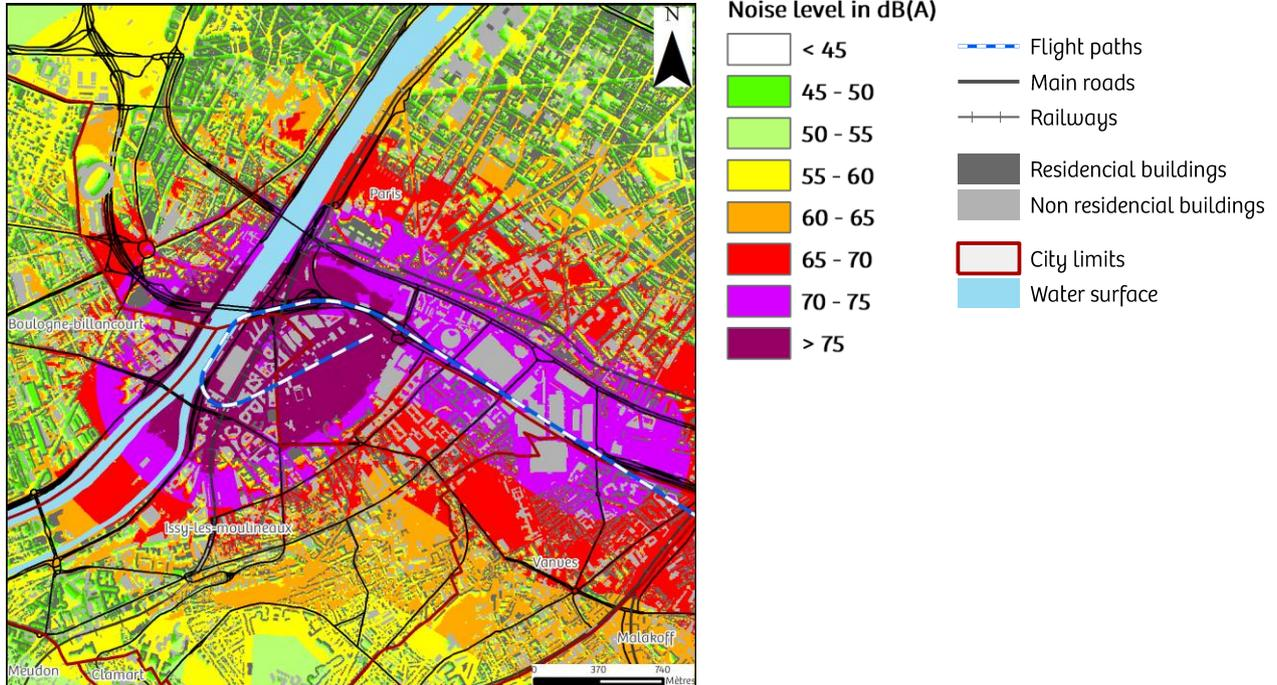
Figure 7 – L<sub>Amax</sub> noise level of the A109 taking-off from QFU06, easterly configuration
