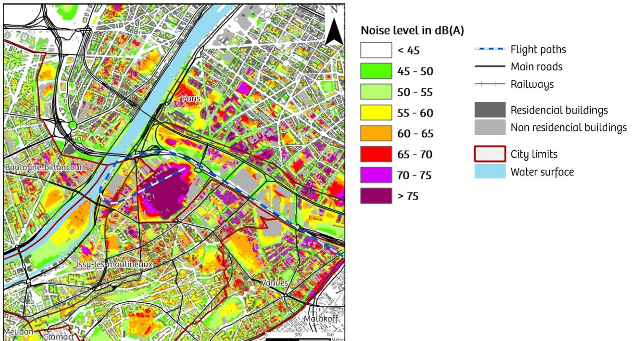
Figure 7 – Noise peaks for the A109 taking-off from QFU06, easterly configuration
