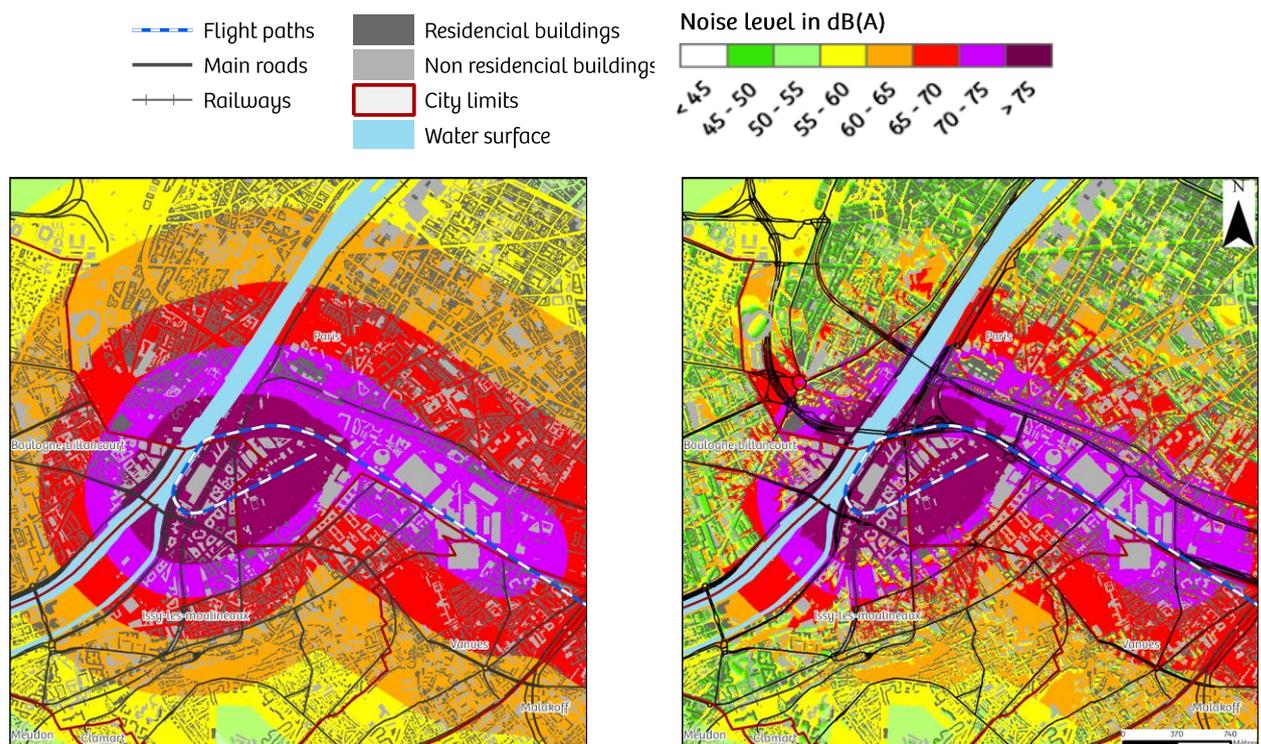
Figures 4 and 5 – L<sub>Amax</sub> noise map generated at ground level by an A109 approaching QFU06, without (figure 4) and with (figure 5) taking into account the effect of buildings
