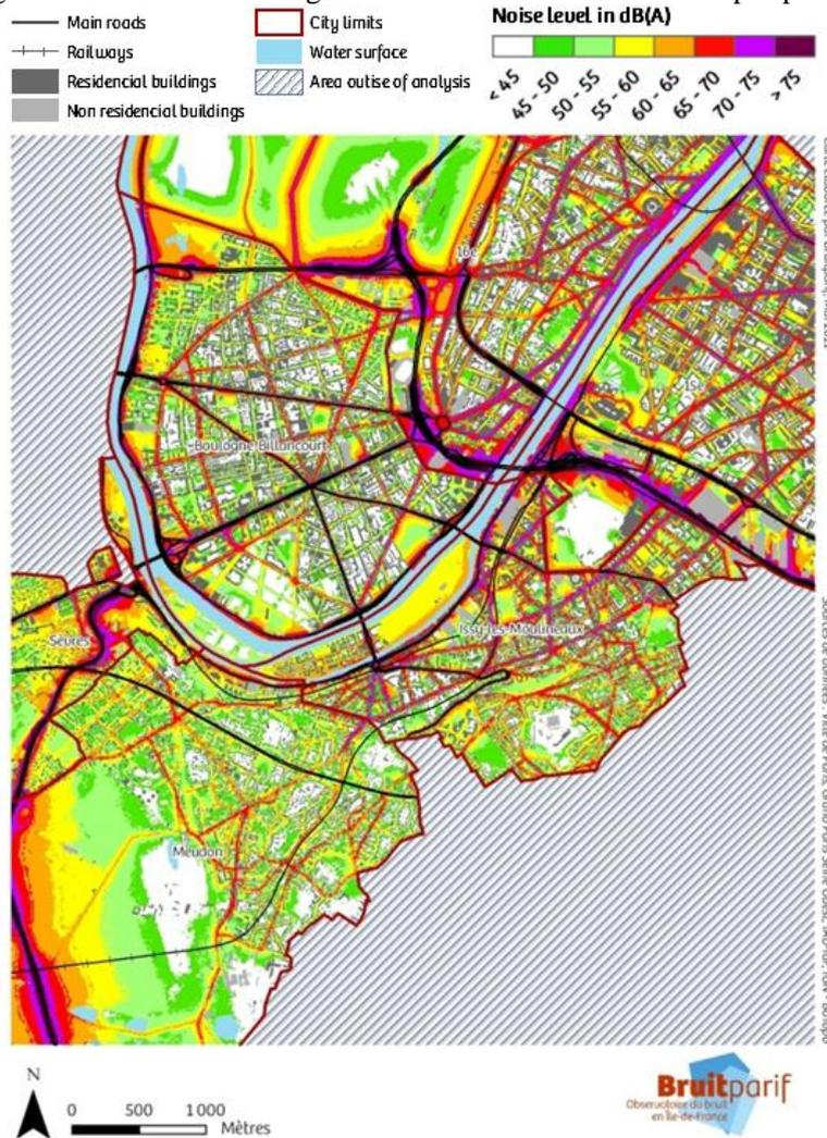
Figure 6 – Road noise map for the LAeq 6 am - 10 pm indicator – Estimation of day-time background noise
